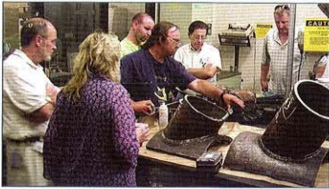
Fig. 6 — Evaluations of test coupons having known defects to develop and validate UT procedure. Witnesses include VMR QA, Level III technicians from both VMR's and Stinger's independent contract inspection services, and Level II inspectors involved in the procedure development.
