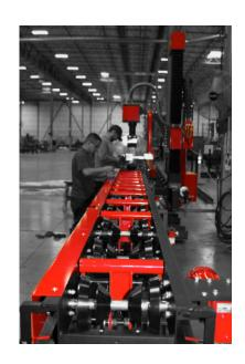
**Gates up** position allows pipe to be rolled from the entrance side onto the conveyor.
