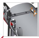
F. Optionally, make beveled end and beginning cuts with the two-torch straight cut-off assembly.
