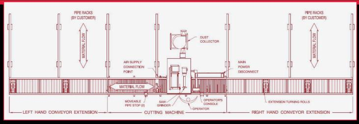
Optional conveyors streamline material flow from either direction.
