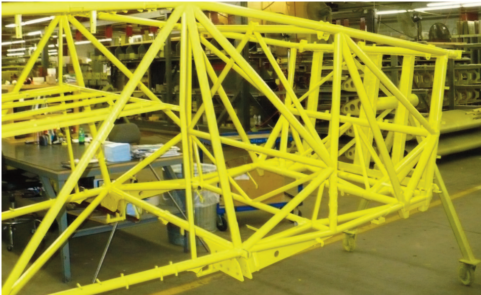
Each fuselage frame is comprised of more than 120 different tube sections.
